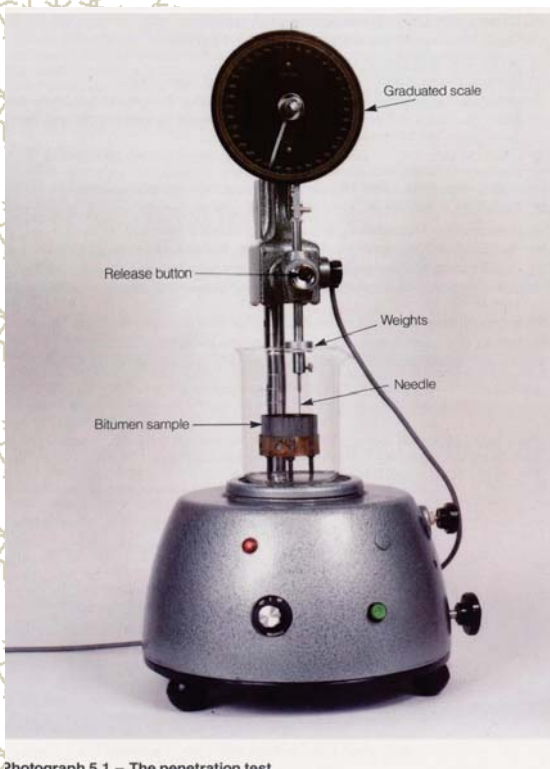
Photograph 5.1 - The penetration test
