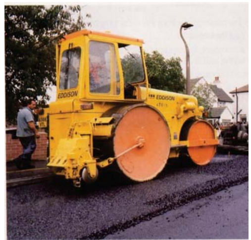
Photograph 13.3 – A traditional deadweight roller
