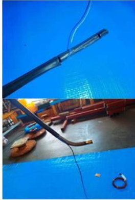
Industrial Endoscope and Thermocouple
