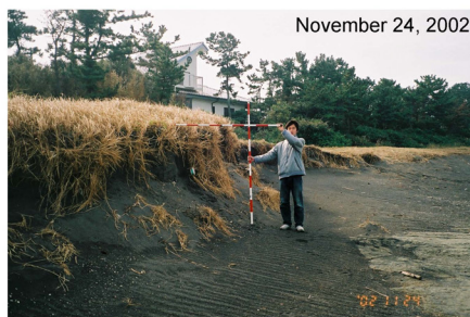
Figure 12. Scarp with 1.6 m height formed in erosion zone (November 24, 2002)
